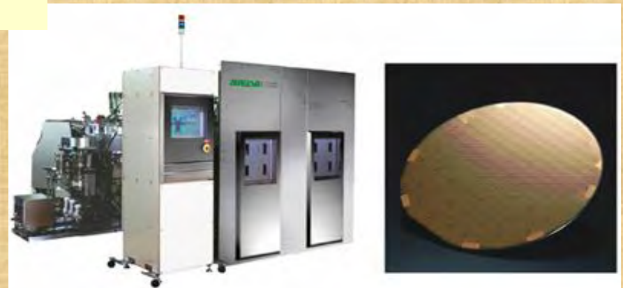
Production deposition system for MgO-TMR devices (Left) A wafer for the MgO-TMR devices (Right)
