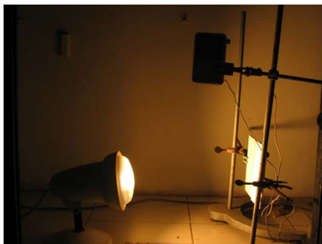
Fig. (2). Experimental setup for measuring the infrared reflectivity of pigments.
